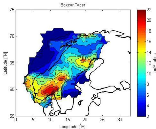
**Figure 6** Spectral displacement amplitude ratios of Lg-waves to P waves.
