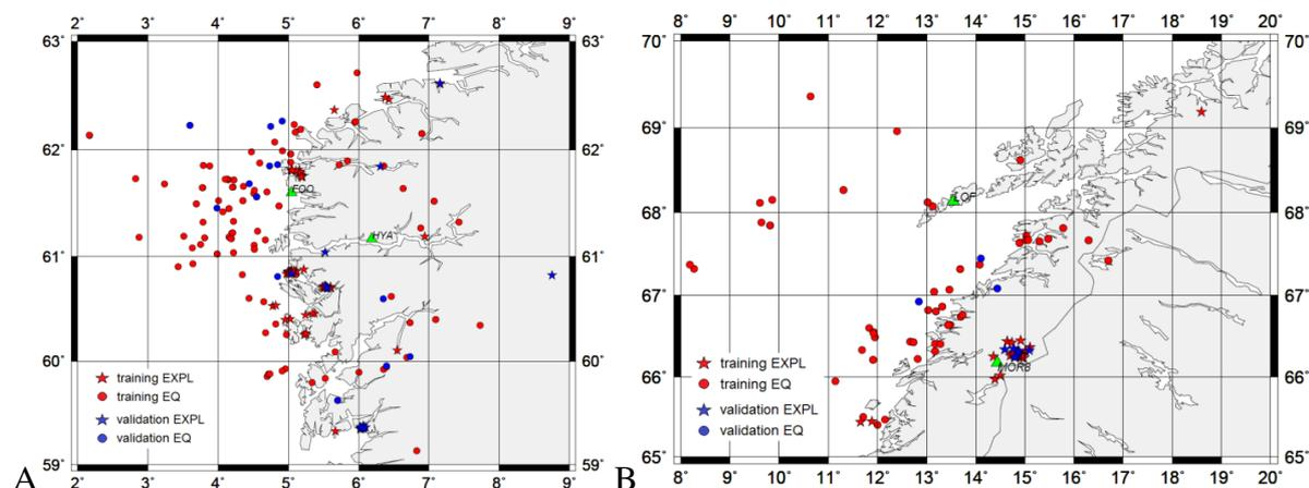
**Figure 9. Seismic events used to develop and verify the reference spectral models for the stations: A) HYA and FOO in the south, and B) LOF and MOR8 in the north. The seismic events are marked as circles and stars, while the seismic stations are marked as green triangles.**
