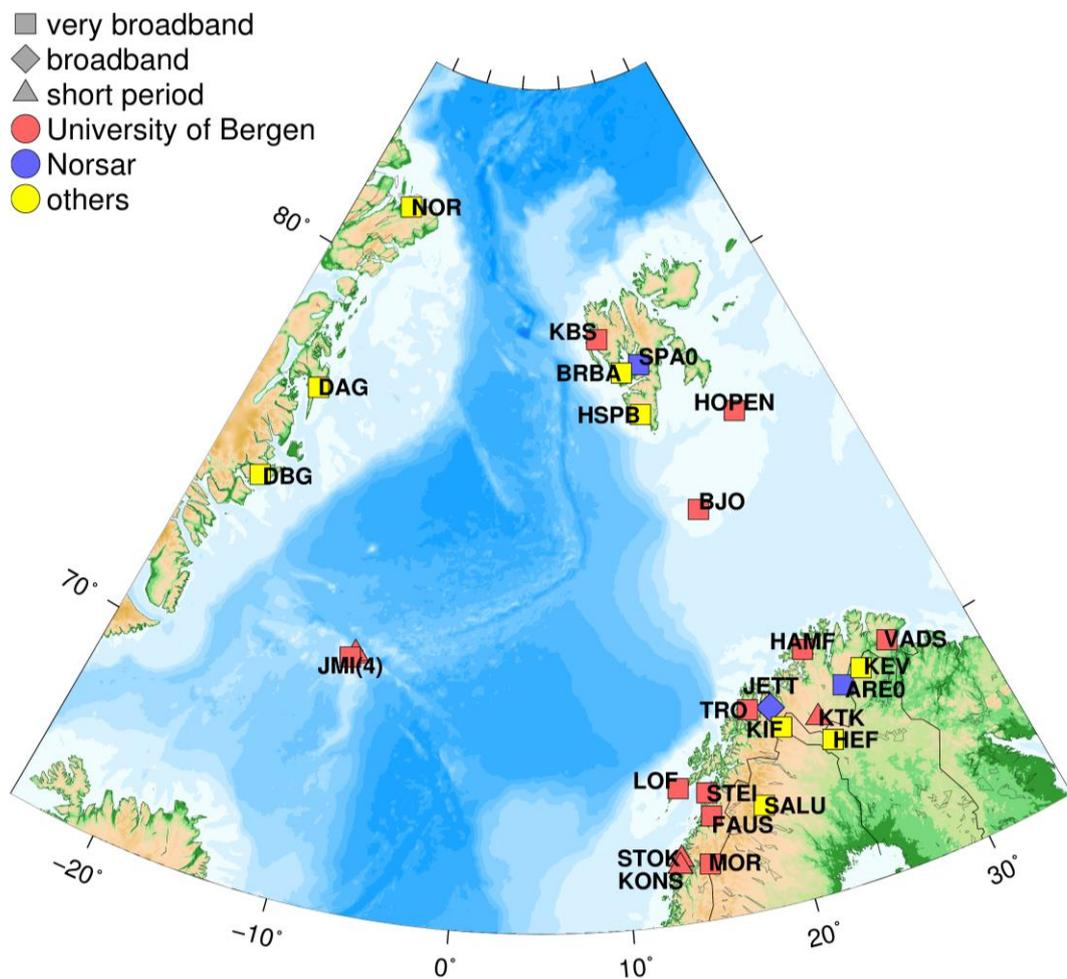
Figure 2. Seismic stations in the arctic area, including the three stations located on Greenland operated by GEUS, Denmark.
