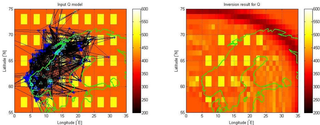
**Figure 7 (a) Synthetic  $Q_{Lg}$  checker board input model with real path coverage (black lines). Light blue triangles represent stations and dark blue stars earthquakes. (b) Inversion result for  $Q_{Lg}$  with the new derived tomographic code.**
