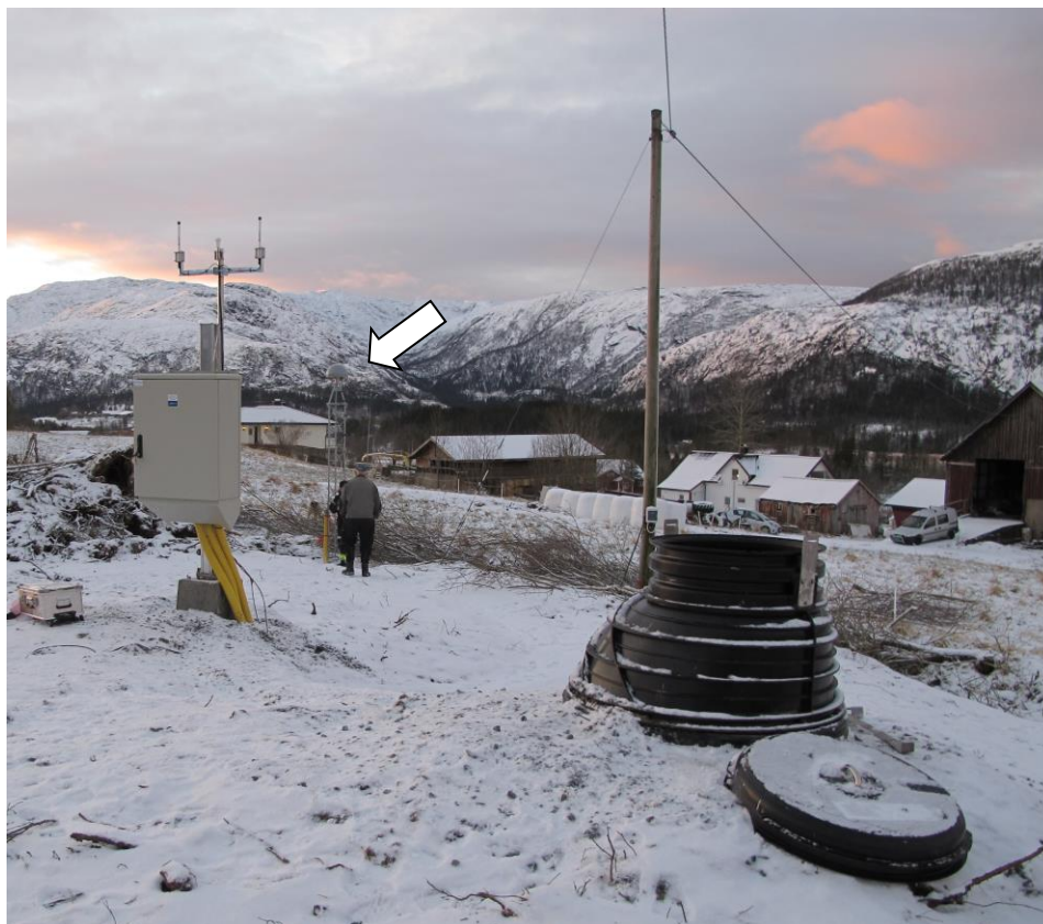
Figure 9. The site for LEIR after completion of the area and installation of the antennas and the connection box. The GSNN antenna mast is marked.
