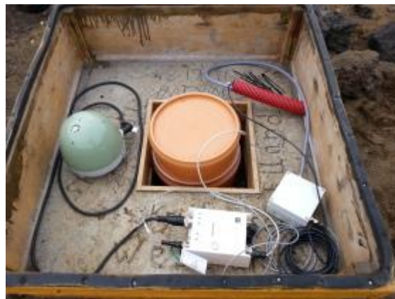
Figure 5. Inside the vault. The trillium sensor (green) is placed at the bottom of the orange plastic tube.
