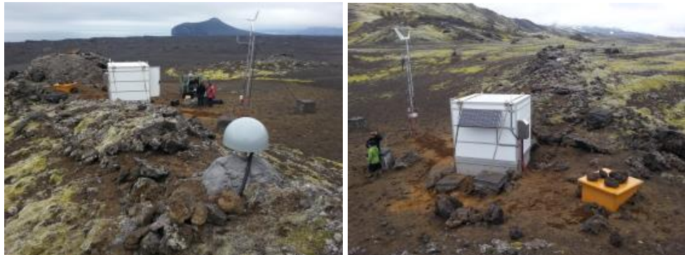
Figure 4 The station JNE after upgrade as seen from two directions: sensor vault (orange), the instrument cabin (white), the GSSN mast and the hemisphere shaped GNSS antenna.
